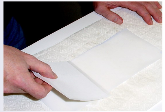
The exceed buffer volume is removed from the membrane
