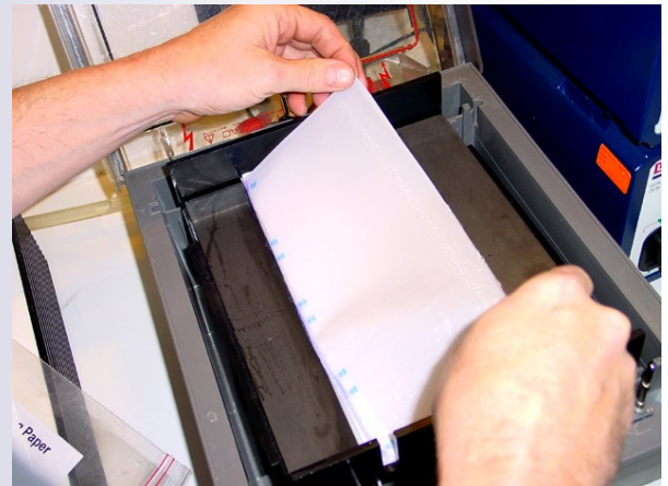
The trans-unit is layed on the anodal blot-stack with the membrane down.
