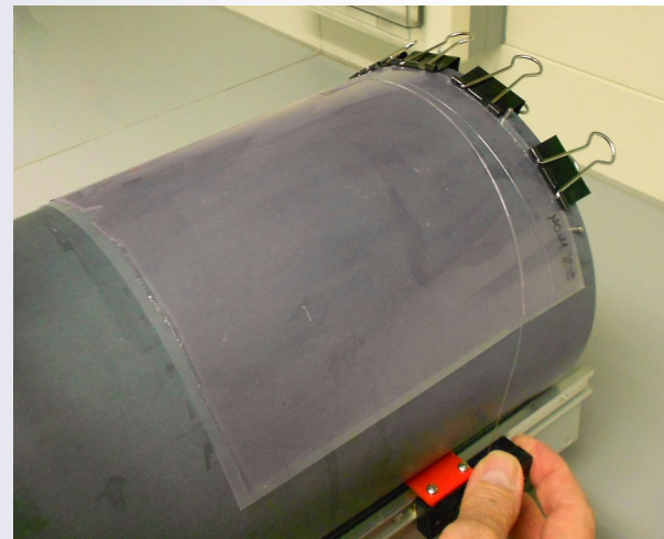
The wire is pulled through the layer: Under the gel and on the support-film!
