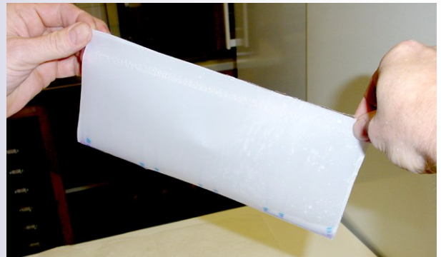
The membrane together with the gel is transported to the blot-stack.
