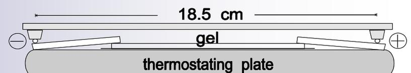
**Fig.8:** Arrangement of gel, buffer and electrodes
