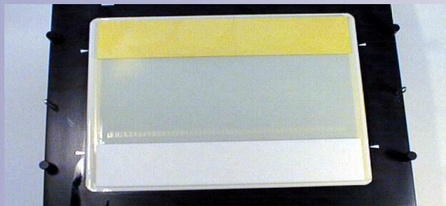
**Fig.6:** flatbed horizontal chamber. Arrangement of gel and electrode strips on the cooling plate.
