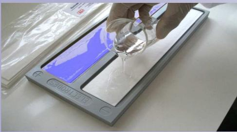
**Fig.5a:** Soak the Electrode Wicks with the electrode solutions
