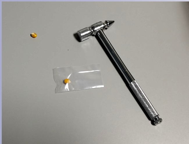
Fig.5: pulverizing a single grain of maize (above) and overlaying with kerosene for defatting (below).
