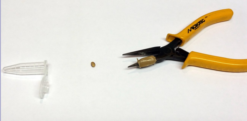
Fig.6: radio pliers for cracking the grain. One side with tape: this prevents splinters splashing out during final grating.
