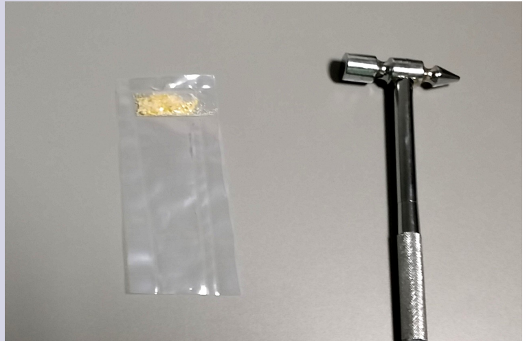
Fig.5: pulverizing a single grain of maize (above) and overlaying with kerosene for defatting (below).
