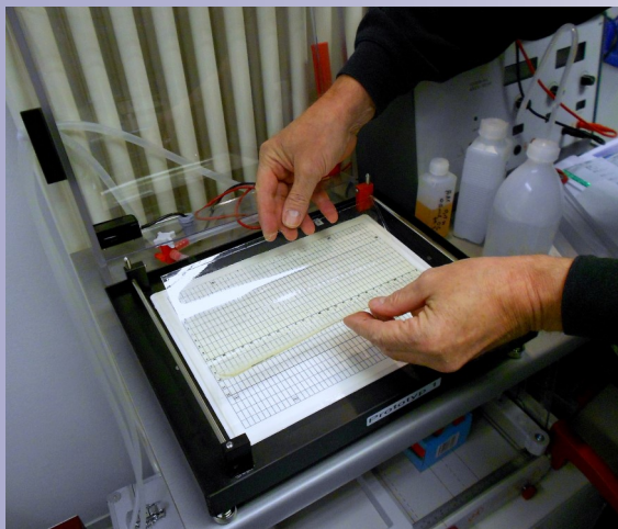
Fig.6: Lowering the bended gel -film down- on the cooling-plate's Kerosene
