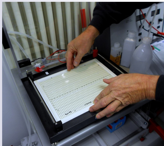
Fig.7: Set the gel down and avoid trapping air-bubble
