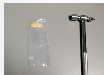
Fig.5: pulverizing single grains of maize (above) and overlaying with ke- rosene for defatting (left)
