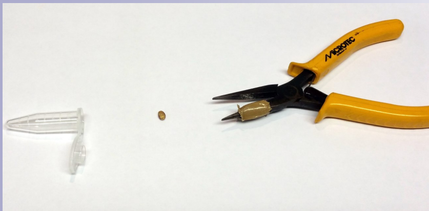
Fig.3a- c: radio pliers for cracking the grain. Philipps-screwdriver for pulverising. One side with tape: this prevents splinters splashing out.
