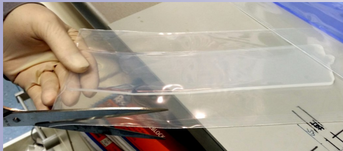
Fig. 5: Cutting out the gel-electrodes out of their bags.
