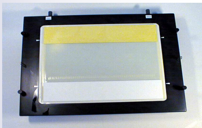
Fig.6: flatbed horizontal chamber. Arrangement of gel and electrode strips on the cooling plate.
