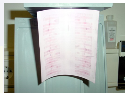
Fig.16: Hanging up the membrane for drying
